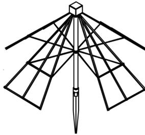
Figure 2: Sketch of an LWA1 tied fork dipole antenna.
