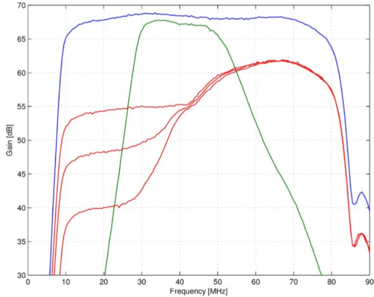
Figure 3: The response of the analog receiver across the passband for each of the three configurations: Full (blue), reduced (green) and split (red). The three red lines correspond to to different attenuator settings of 6, 12 and 20 dB respectively.
