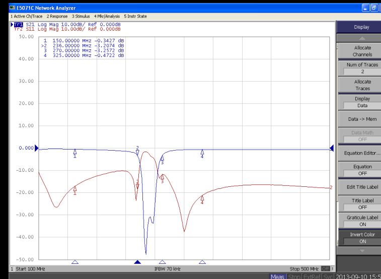
Satellite Notch Filter (236-270MHz)
