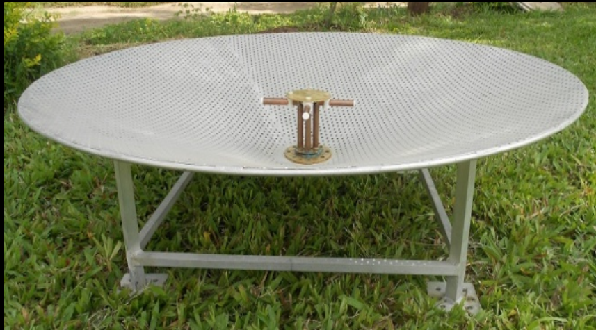
Cone Dipole design (for 550-900)
