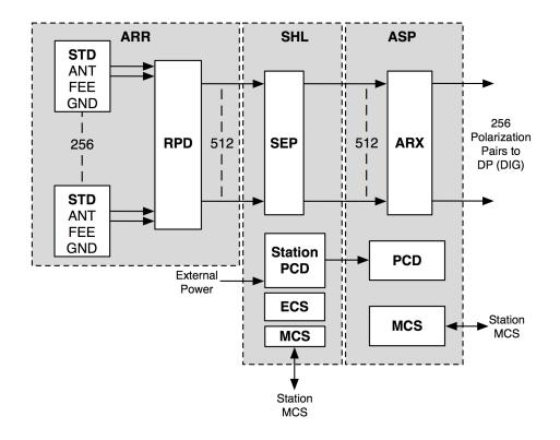
Figure 1: Station architecture: antennas through analog receivers.
