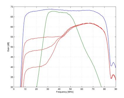
Figure 7: Magnitude response of the ARX in full-gain configurations for each of the 3 filter settings. Split Bandwidth attenuator settings (red) at 6 dB, 12 dB, & 20 dB down.
