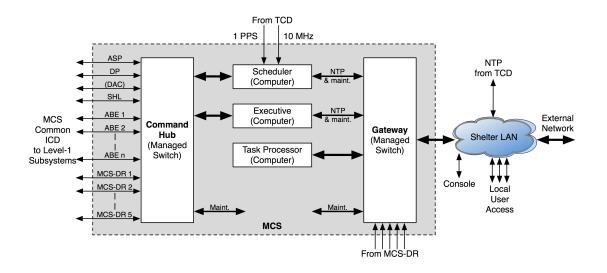
Figure 4: Station monitoring & control architecture.
