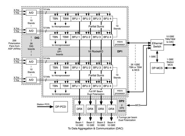
Figure 2: Station architecture: digital processor. "GBE" is Gigabit Ethernet.
