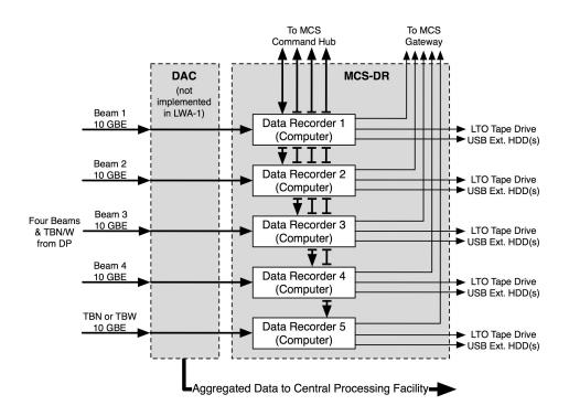
Figure 3: DAC and MCS Data Recorders. For LWA-1, the MCS-DR will be implemented. For subsequent stations, the DAC will be implemented.
