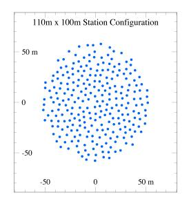
Figure 6: Pseudorandom elliptical array geometry [35].
