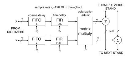
Figure 8: Beam Submodule. Each incoming sample is w = 12 bits wide, and the partial sums are w + 8 = 20 bits wide.  $D_x$ ,  $D_y$ ,  $d_x$ , and  $d_y$  are control numbers; P is a 2x2 coefficient matrix; and L, F,  $b_f$  are filter design parameters.
